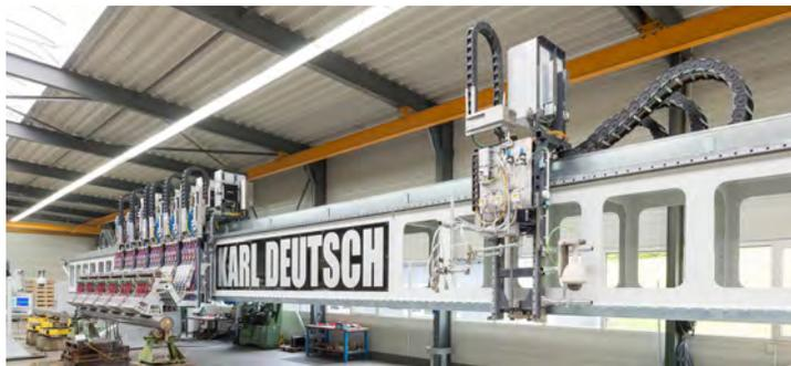
Additionally, EKD equipped the chains with sliding elements on the inner radius to reduce driving forces. This chain model ensures smooth and precise force and motion transmission, ensuring reliable testing operations in the long run.
